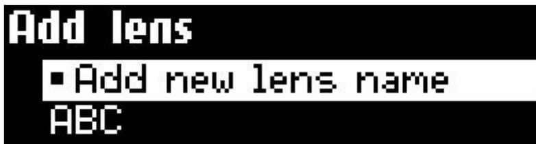
To add a new lens name, use the joystick up/down to scroll through the available characters. One click for a single increment, hold for rapid scroll. Click right to type the next character.
