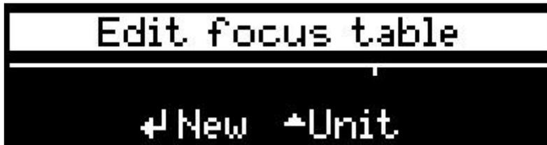
Set the units of measurement for focus by pushing the joystick UP. Choose metres or feet.
